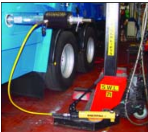
◀ An RACH-602, powered by a P-392 handpump, is used to extract corroded carriage pins from refuse collection vehicles.
