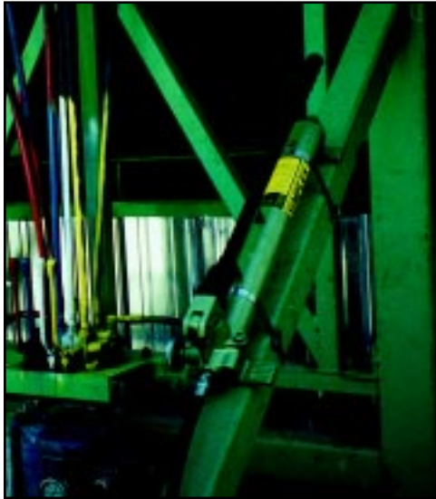
This forms manufacturer uses Simplex hand pumps and cylinders mounted to the structure for fine positioning. "We needed a hand pump that was easy to use and reliable." Simplex P41 hand pump is the preferred choice.
