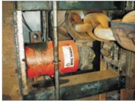
PE4004S pump and RD3006 cylinder used in a special press which repairs damaged chain links.
