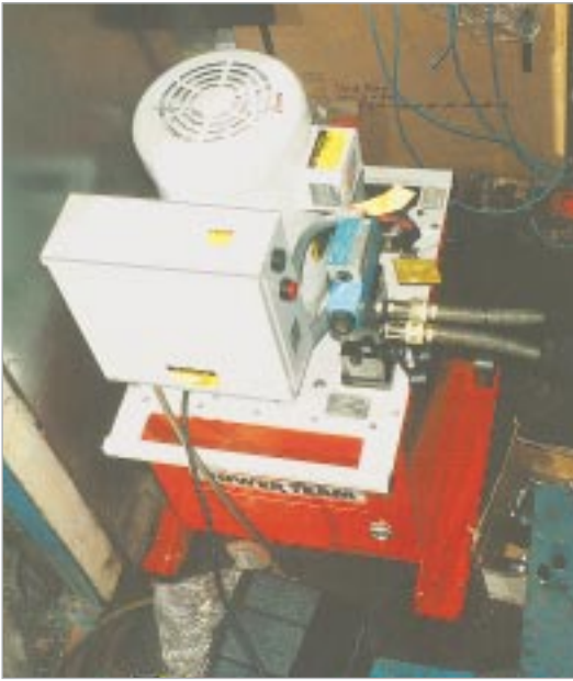
PE4004S pump and RD3006 cylinder used in a special press which repairs damaged chain links.
