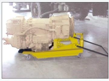
The TTJ3 Transmission Jack (NSN 4910-01-396-5044) with its new TTJ-Z1FA Lifting Saddle Assembly easily handles the massive Allison MD 3070 PT transmission with its offset transfer case for the militarys new FMTV vehicles. Technicians can now work safely with the MD 3070 PT without being forced to remove any vehicle components or raise the FMTV.
